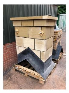
courses down from the top of the brick work. These lifting lugs are designed to be attached using lifting shackles. Once lifted and fixed into position the lifting lugs can then be removed and the bolt pushed through into the stack, the holes should then be filled with an external quality sealant and over pointed.
