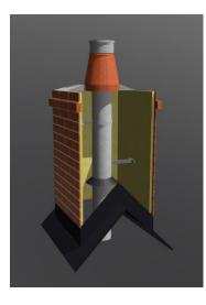
Our chimney stacks can be adapted for either preinstallation of flue lengths or for on site installation of a flue system. If you intend on using a flue within the stack, please confirm at the time of order so we supply an open chimney pot rather than a fully sealed closed pot on our "dummy" stacks.
