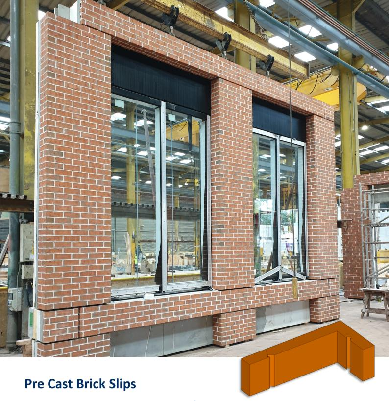
Fab-Lite Pre-Cast brick faced cladding gives a building the appearance of being traditionally built—but the use of factory methods offers advantages in terms of design, quality and speed.
